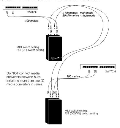
Recessed switches located on each side of the media converter are used to configure the media converter for the network. NOTE: Switch labels are located AT TOP of C/E-R-TX-FX-01 media converter.
